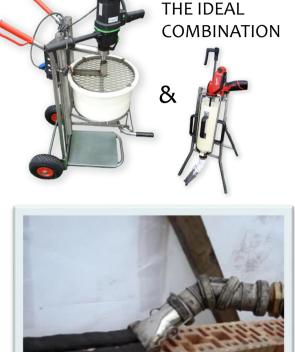
The Gema©k Mortar Processing System used for exterior walls is also very good for interior walls made of Poriso, Porotherm and other similar inner wall bricks/blocks. Using standard glue or thin bed mortar for outer walls, where the joints can be just 3 to 8 mm thick,
